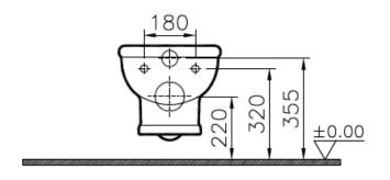
Additional pipe may be required as to wall thickness.
