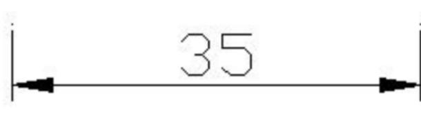
A horizontal dimension line with arrows at both ends, indicating a width of 35 units. The number is oriented horizontally.
